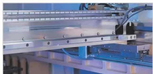
Linear Motor driven XY gantry for faster and more accurate production
